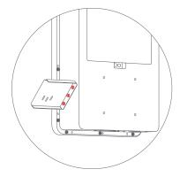
• Fix the POS mount bracket with three M4 machine screws on the right side of device's main body;
