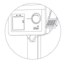
Method (2): Connect the POS cable using separator and insert into column bracket's opening; one-end connect to device's main body, another end connect to the power supply.
