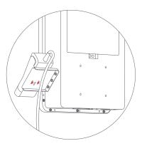
2 Install the POS terminal, fix the terminal back using two M3 machine screws, connect the wiring cables.
