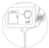
Method (1): Connect the POS cable using separator; one-end connect to device's main body, another end connect to the power supply.
